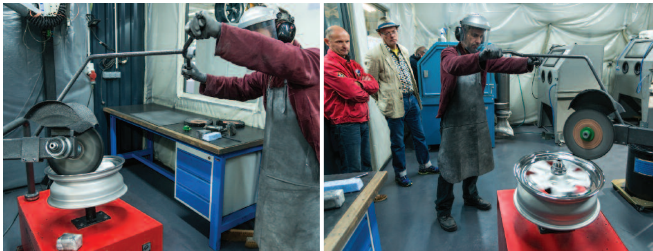
More specialist machinery, this time to polish the outer rim. Patrick Pugin insists on a 'clean air' environment, with extractors to remove any contamination
