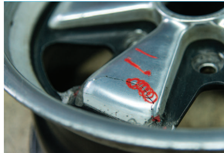
A cracked rim like this can be repaired. Right: It's not all about the wheels. The Art Restoration side of Patrick's business handles complete classic Porsche restorations
