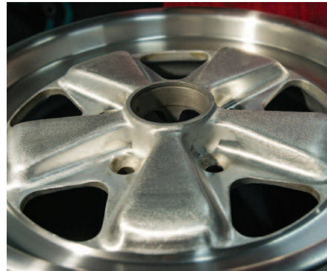
Anodising is a chemical process involving a nitric acid bath and an electric current, which causes oxidation of the surface of the metal
