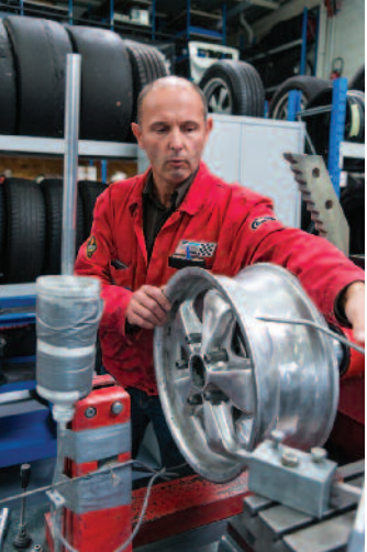
Below left to right: Patrick first checks each wheel for run-out, straightening the rims as necessary; blasting removes all traces of the original paint; huge polishing machine is manually manoeuvred into position against spinning wheel
